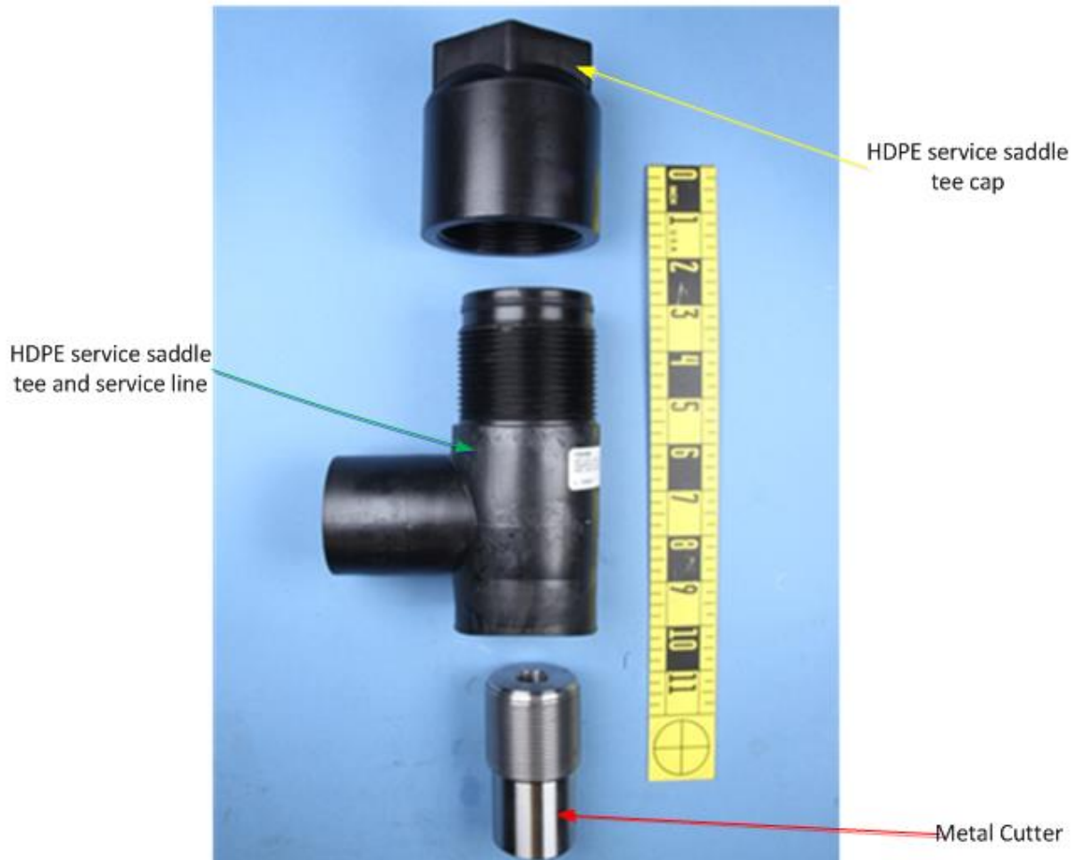
Figure 5: Gas service saddle tee components showing HDPE cap, saddle tee and metal cutter
