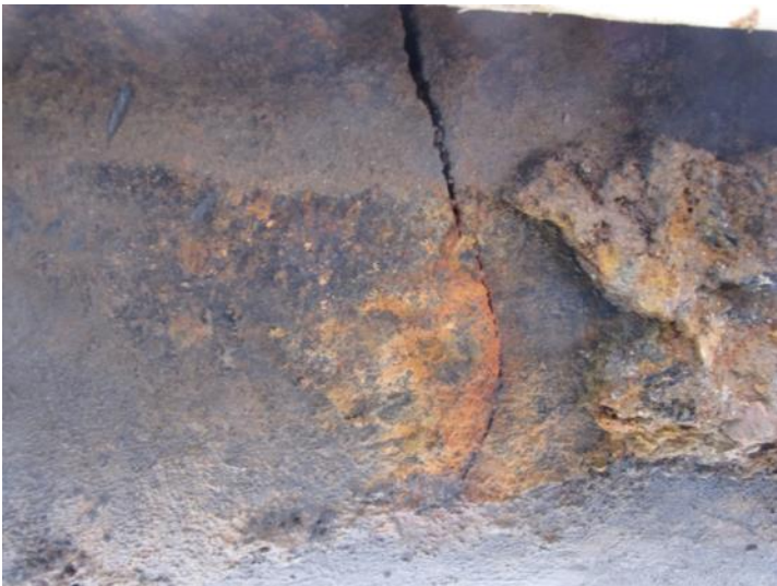
Figure 16: 12-inch water main pipe with circumferential crack bottom view.
